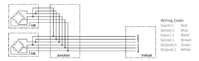
Depending on the application the junction box should be protected to at least IP54 (DIN.40.050), but for wash down purposes we strongly recommend a junction box protected to IP65. The degree of protection can only be achieved if the junction box is installed correctly:
